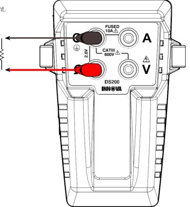
Figure 4: Resistance Measurement
