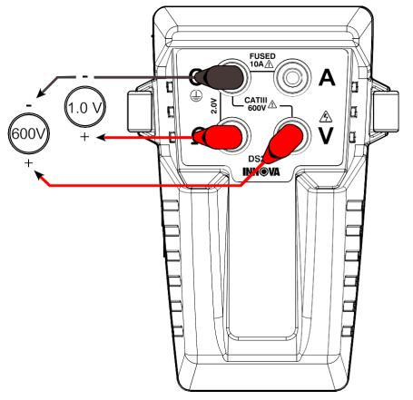
Figure 1: Basic Voltage Measurement
