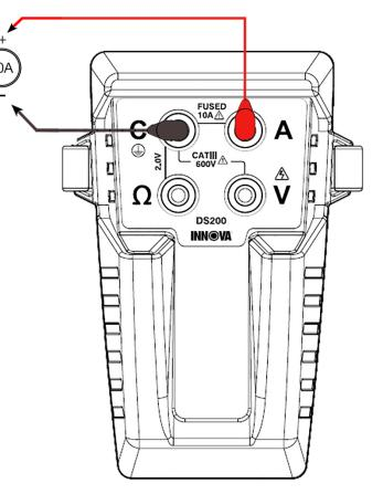
Figure 2: Basic Current Measurement
