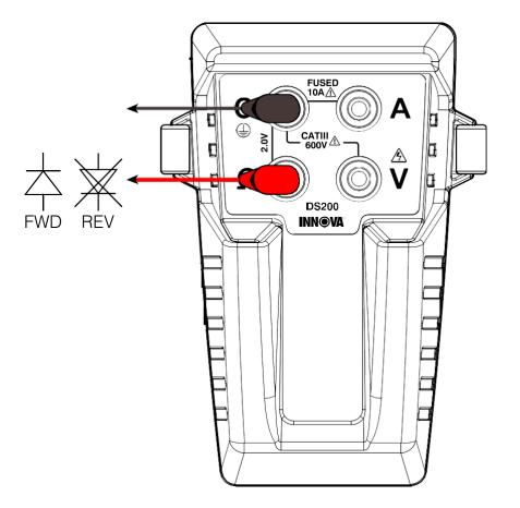
Figure 5: Diode Measurement
