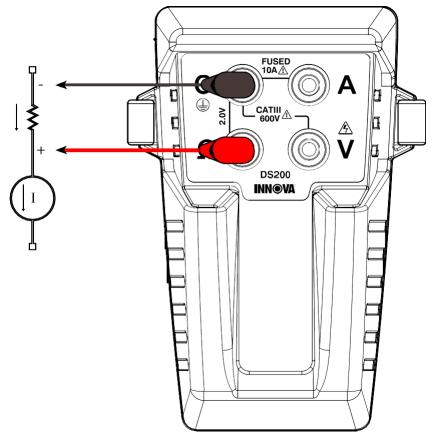
Figure 3: External Current Shunt
