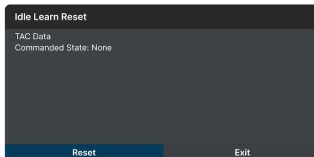
5. A “results” screen displays when the reset procedure has been completed. Tap **Exit** to terminate the procedure.
