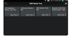
Request Control On-Board System - \$08 – Enable the external test equipment to control the operation of an on-board system, test, or component.
