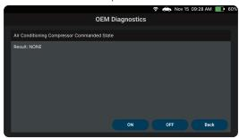
**4.** Tap the appropriate **control** to operate the actuator as desired.
